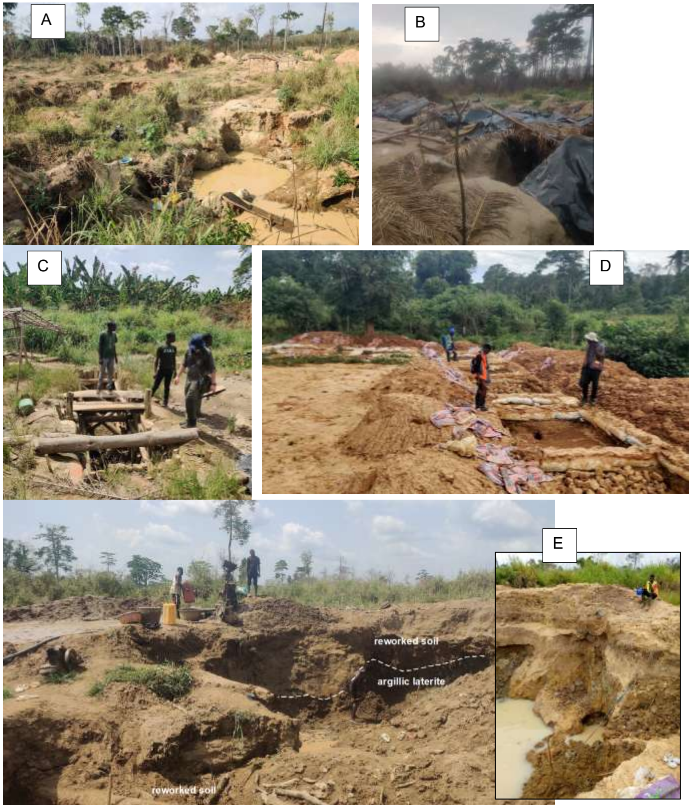
Figure 6-6 - Artisanal miners' activity in the project area at March 2023. A: washing and excavation facility, soil and saprolite. B and C: shafts and trenches to mine quartz veins (depth of 15-20 m); D: Artisanal cyanide leaching tanks. E: washing with a mechanised tool. Note the thickness of reworked soil.
