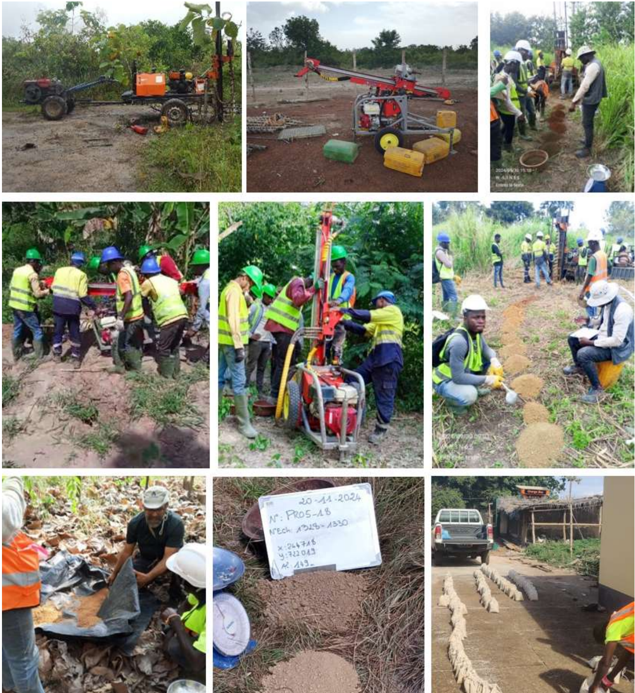
Figure 9–9 Several phased of the auger drilling campaign with heavy and light rigs; sampling and logging, and physical inspection prior to shipment to the lab.
